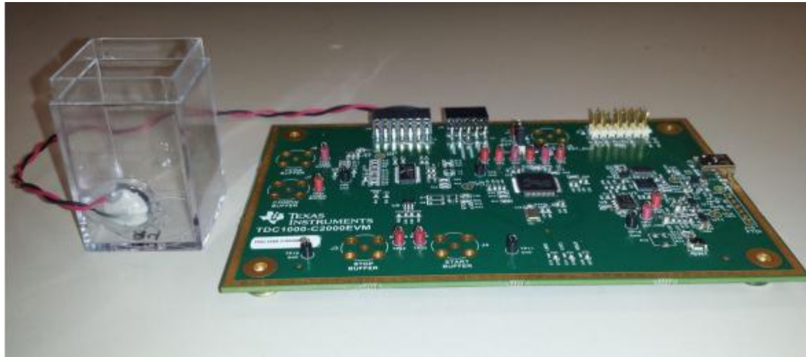
TDC1000-C2000 EVM with Test Cell to Measure Concentration
