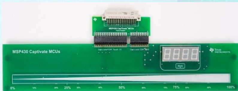
4 IOs = 12 inch slider, 1/100 th inch accuracy
