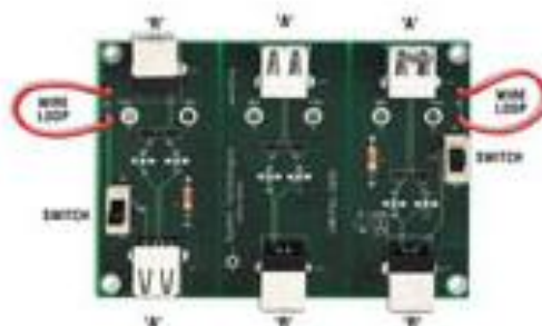
E2646A SQiDD fixture •FS/LS Signal quality, Inrush
