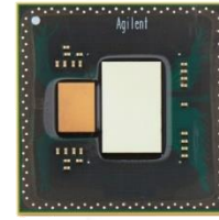
65 nm CMOS ADC with 130 nm Bi-CMOS buffer IC
