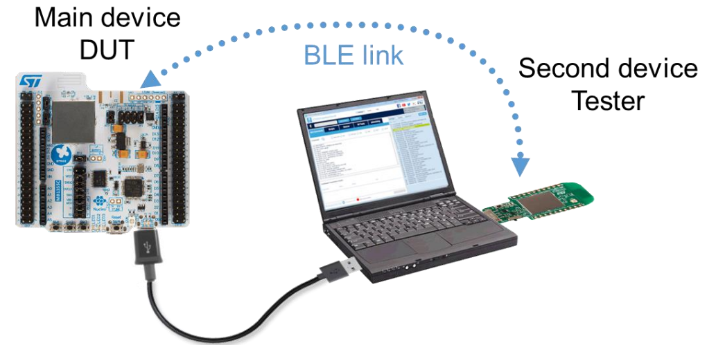
RF test with two devices
