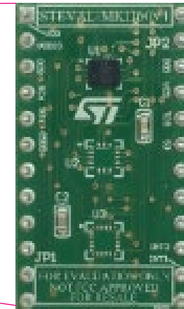
Sensor adapter board for a standard DIL24 socket
