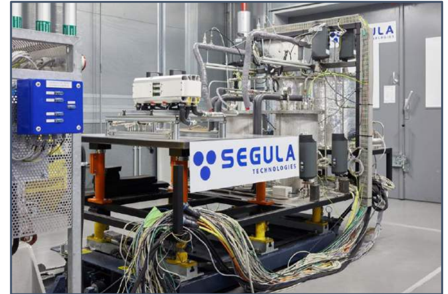
A hydrogen fuel cell stack on a test rig in the SEGULA lab. (Image credit: SEGULA Technologies)
