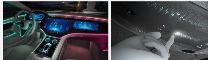
Dynamic animations and HMI extension done via ECU to control multichannel UARToverCAN RGB LED drivers
