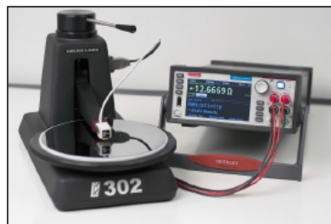
Figure 1. Model 2450 SourceMeter SMU Instrument with the Lucas/Signatone Corporation (Gilroy, CA) Model SP4 4-Point Probe Head and S-302 Test Stand measuring the resistivity of a sample.
